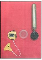
When examined the above component satisfied the relevant requirements of the technical specification EN ISO 12402-7:2007+A1:2011, Clause 4.11 and Table 18 for manual inflation systems for hybrid and fully inflatable PFDs.
