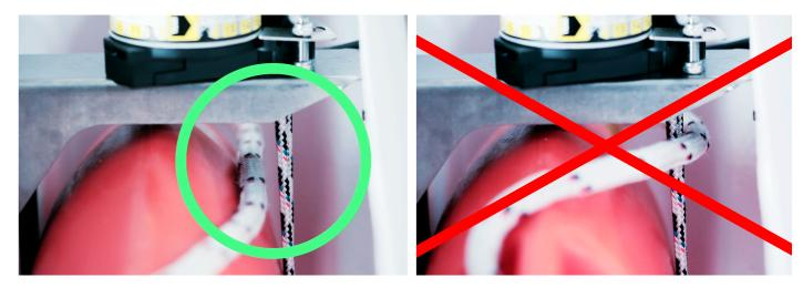
5. Pull up the release cord through the ERU hole with the pilot line. Secure it with the manual safety pin.
