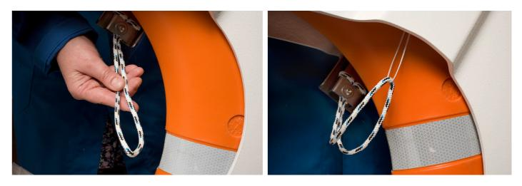
Make sure that the lifebuoy line is not on the outward side of the release cord! This might entagle the lifebuoy in an activation situation.
